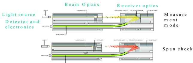
Diffuser creates scatter in span check
