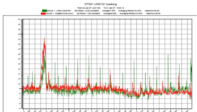
3. The PCME QAL 991 and PCME QAL 181 have dissimilar results during plant stop and start up when there water condensation issues. This issue appears to be related to the different effects of water vapour on both instruments
