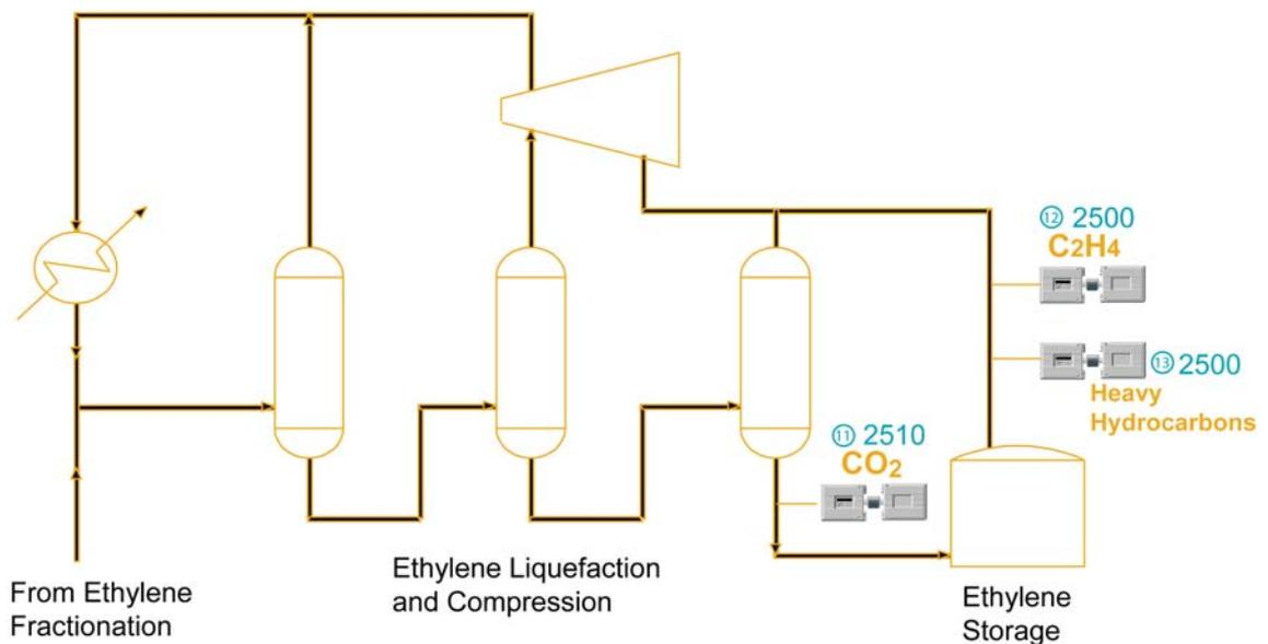
⑪ ⑫ & ⑬ The ethylene product at the end of the process is monitored for residual CO<sub>2</sub> traces to check purity. The ethylene purity is also measured (99.9%), and the level of any heavy hydrocarbons.
