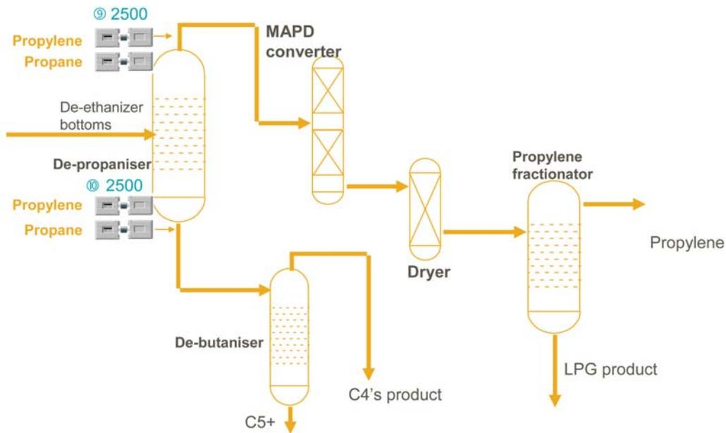
⑨&⑩ The de-propaniser separates C3's and C4's+. Then the propane is separated from the propylene in a fractionator. The de-propaniser bottoms are then sent to the de-butaniser to separate the C4's from C5's+
