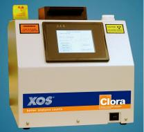
inorganic, and total chlorine using the CLORA analyzer. This is important because although most of the inorganic chlorine in crude oil coming into a refinery is effectively removed by the desalter, organic chlorides will stay with the crude and downstream processing can break them down into hydrochloric acid which may in turn cause corrosion issues.
