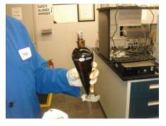
Put 25 ml of crude into a separatory funnel. Add 75 ml of hot DI water. For solvent diluted crudes, use 50 ml of crude/solvent mixture to 150 ml hot DI water. Cap the separatory funnel and shake vigorously for two minutes. Periodically degassing the sample by venting the cap will prevent gas buildup.
