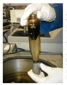
Put 25 ml of crude into a centrifuge tube. Add 75 ml of hot DI water. Different amounts of crude and water may be used, but the 3:1 water/hydrocarbon ratio is recommended for effective extraction. Cap the centrifuge tube and shake vigorously for two minutes. Periodically degassing the sample by venting the cap will prevent gas buildup.
